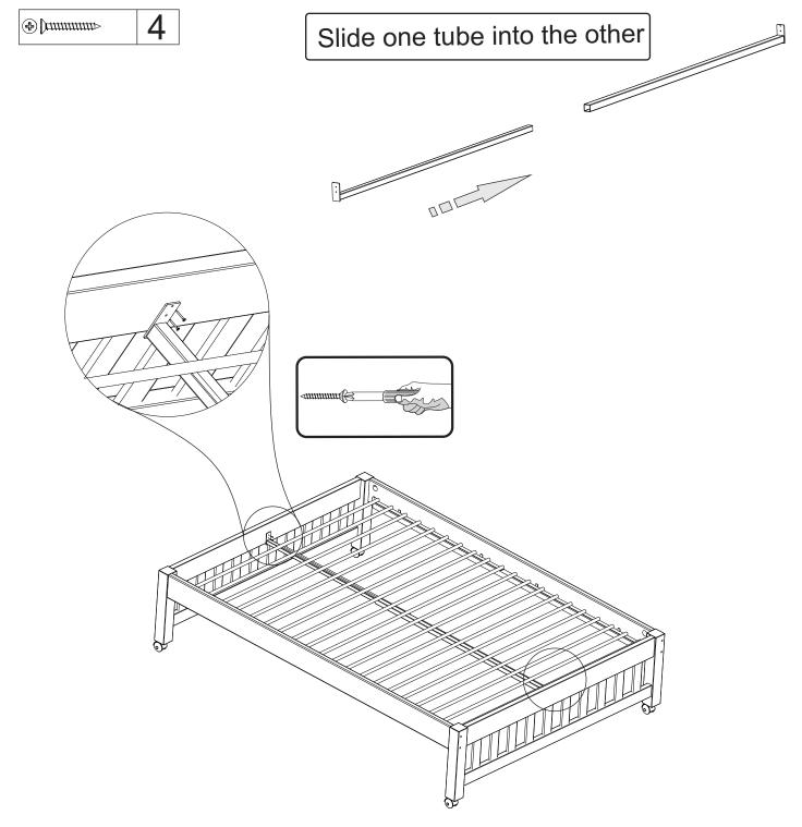
Hold the center support under the slats, center it on the bed and screw it on both sides using the screws supplied
